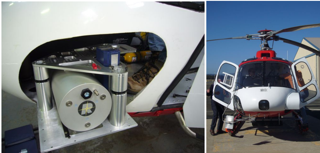
(a) The laser mount installed in the front left floor window of the helicopter. (b) The cowling over the laser mount in the front left floor window.
